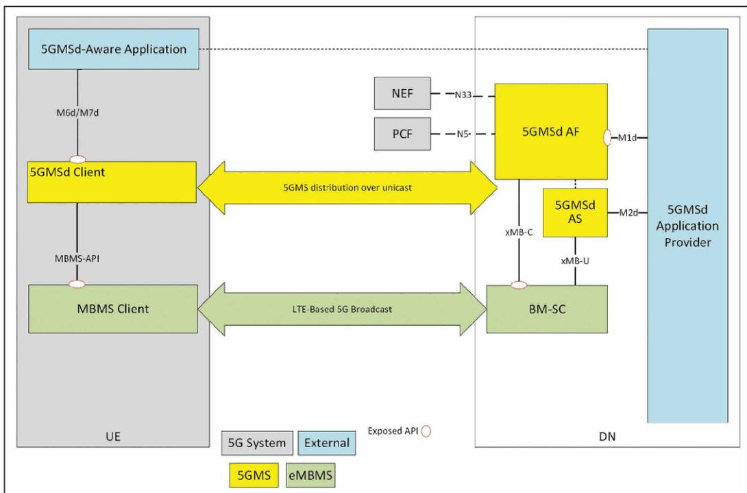
FIGURE 2. Option 1: 5G Broadcast capabilities used by 5GMS.
